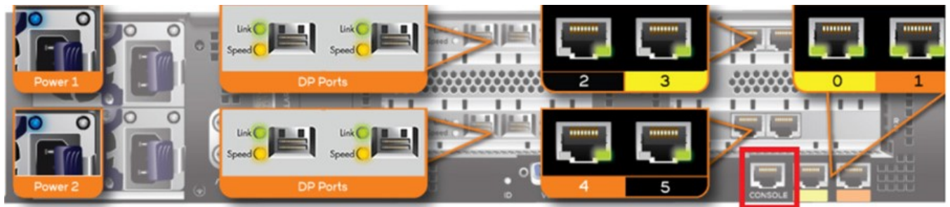
FIGURE 2 SZ300 Location of console port
