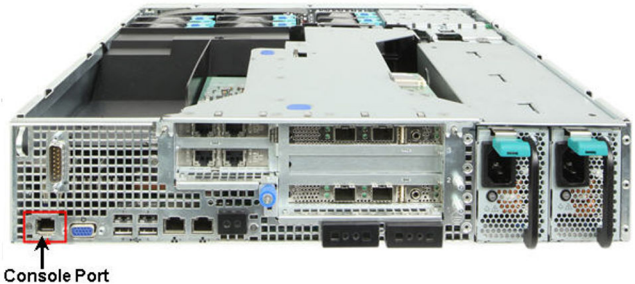
FIGURE 2 SZ300 Location of console port
